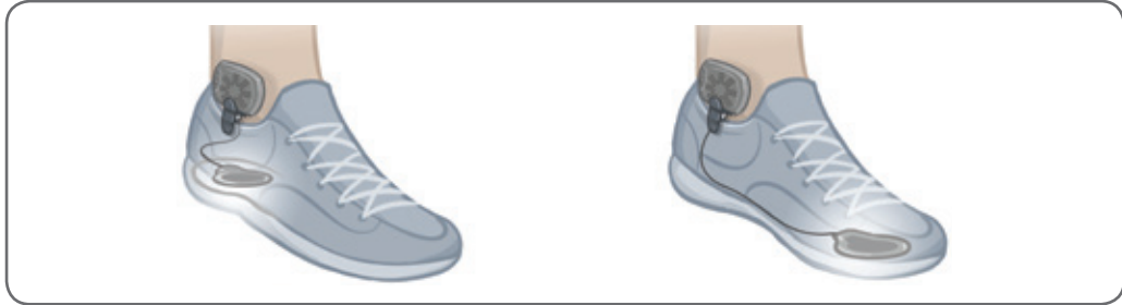
Figure 6-19: Final Position of the Foot Sensor Attached to the Shoe
