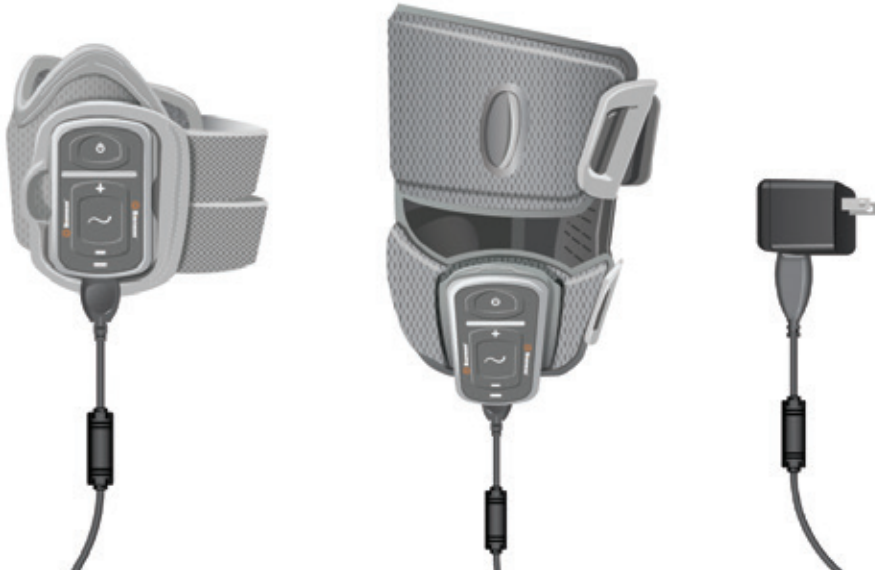
Figure 6-2: L300 Go System Charging Setup (Example of a Lower Leg FS Cuff and Thigh Cuff Configuration)
